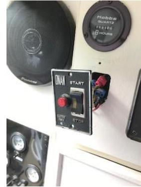
*With a small modification to the wiring on the back of the Onan panel I was able to accomplish this. There are also 4 wires that need to be connected together at the generator for the remote panel connection. The wiring connections are as follows:*
